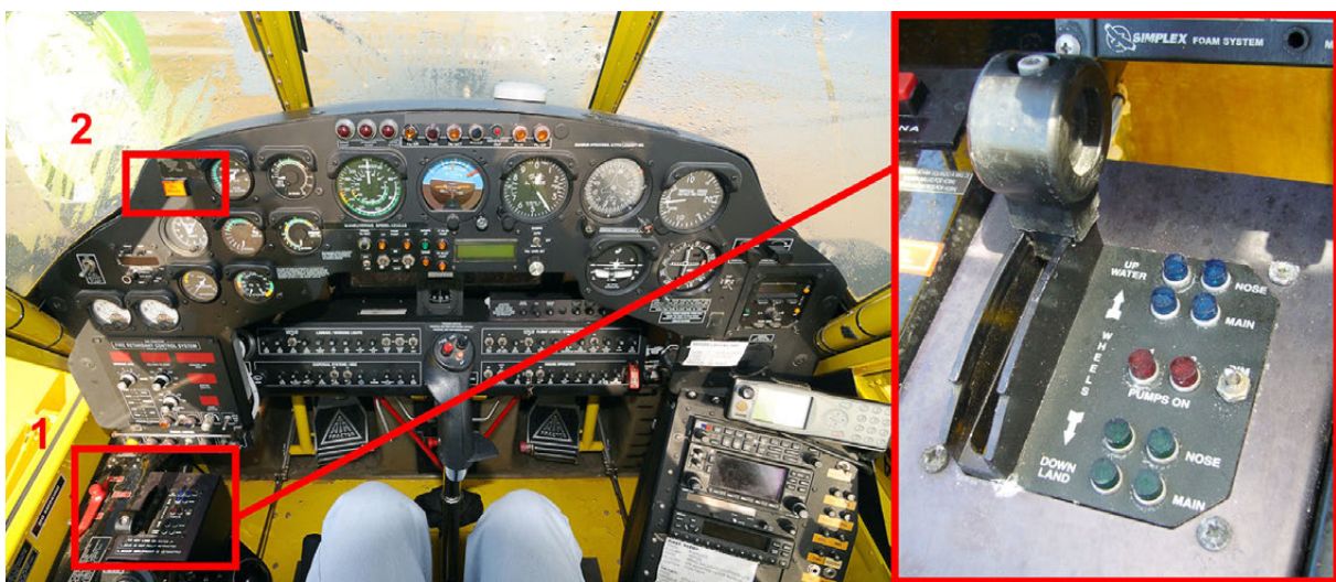
Figure 2. Location of visual gear indications in the cockpit of the AT802A
